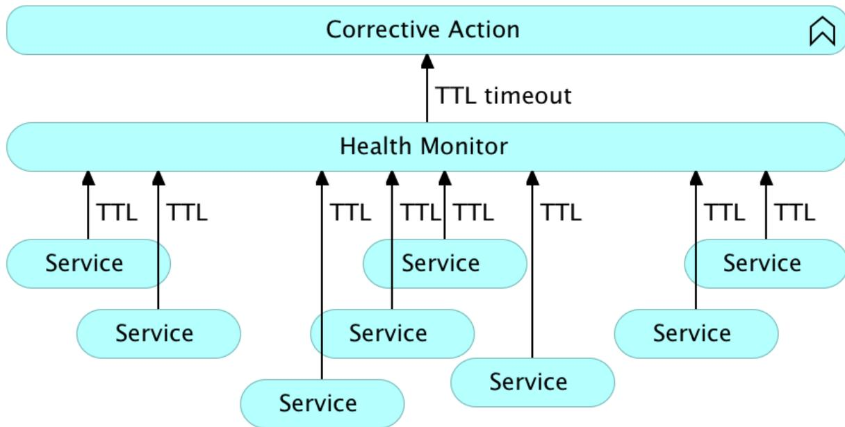
Figure 15-01: System level self-healing with time-to-live (TTL)
