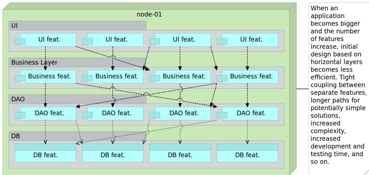
Figure 3-2: Monolithic application with increased number of features
