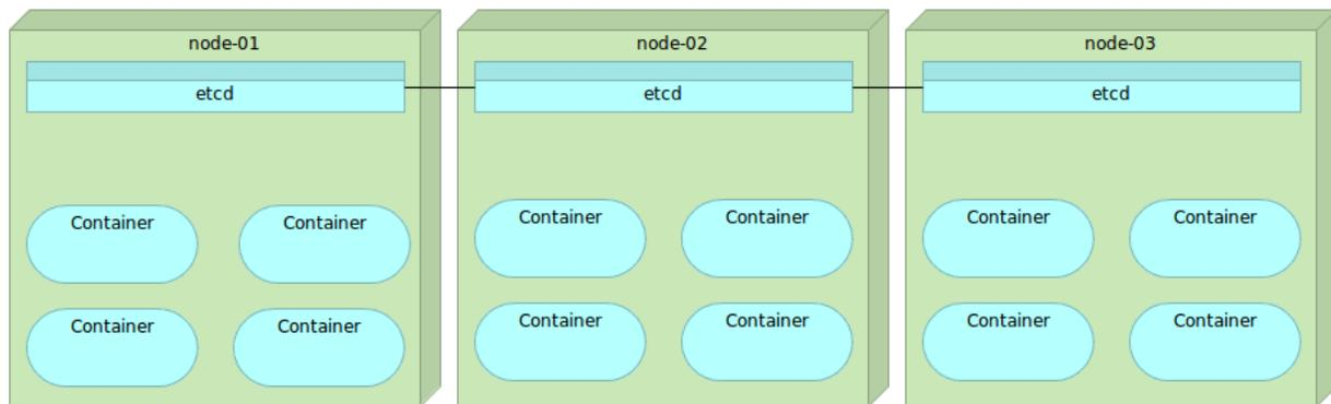
Figure 8-6: Multiple nodes with Docker containers and etcd
