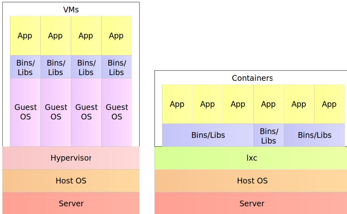
Figure 2-8: Virtual machines and containers resources utilization comparison
