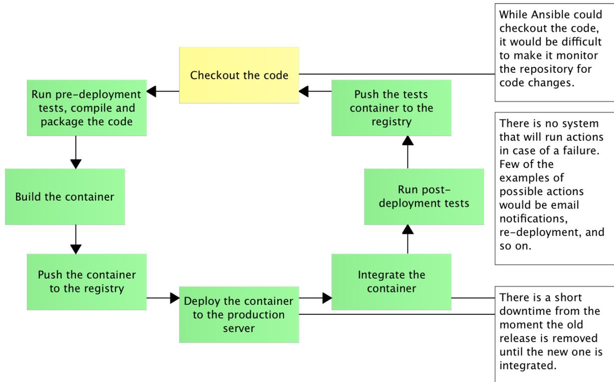
Figure 11-4: Missing pieces in the deployment pipeline
