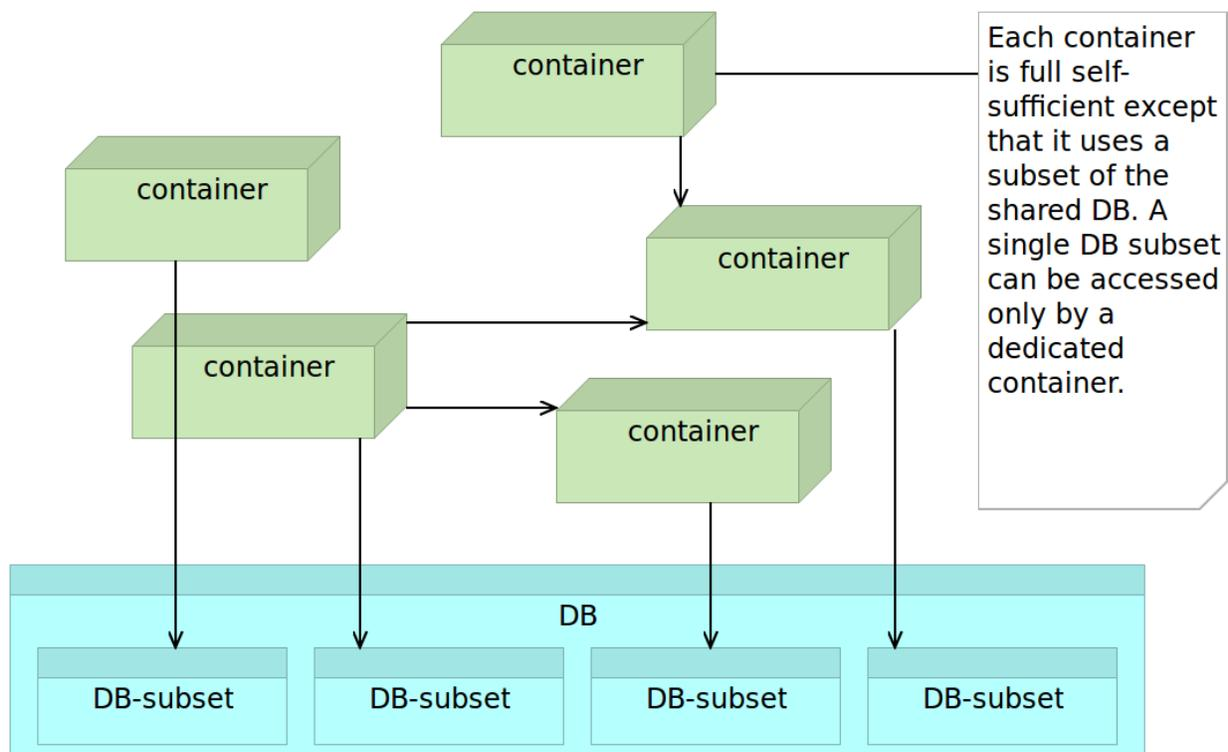
Figure 3-16: Microservices inside containers accessing the shared database
