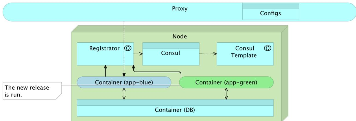
Figure 13-8: The green container is deployed in parallel with the blue
