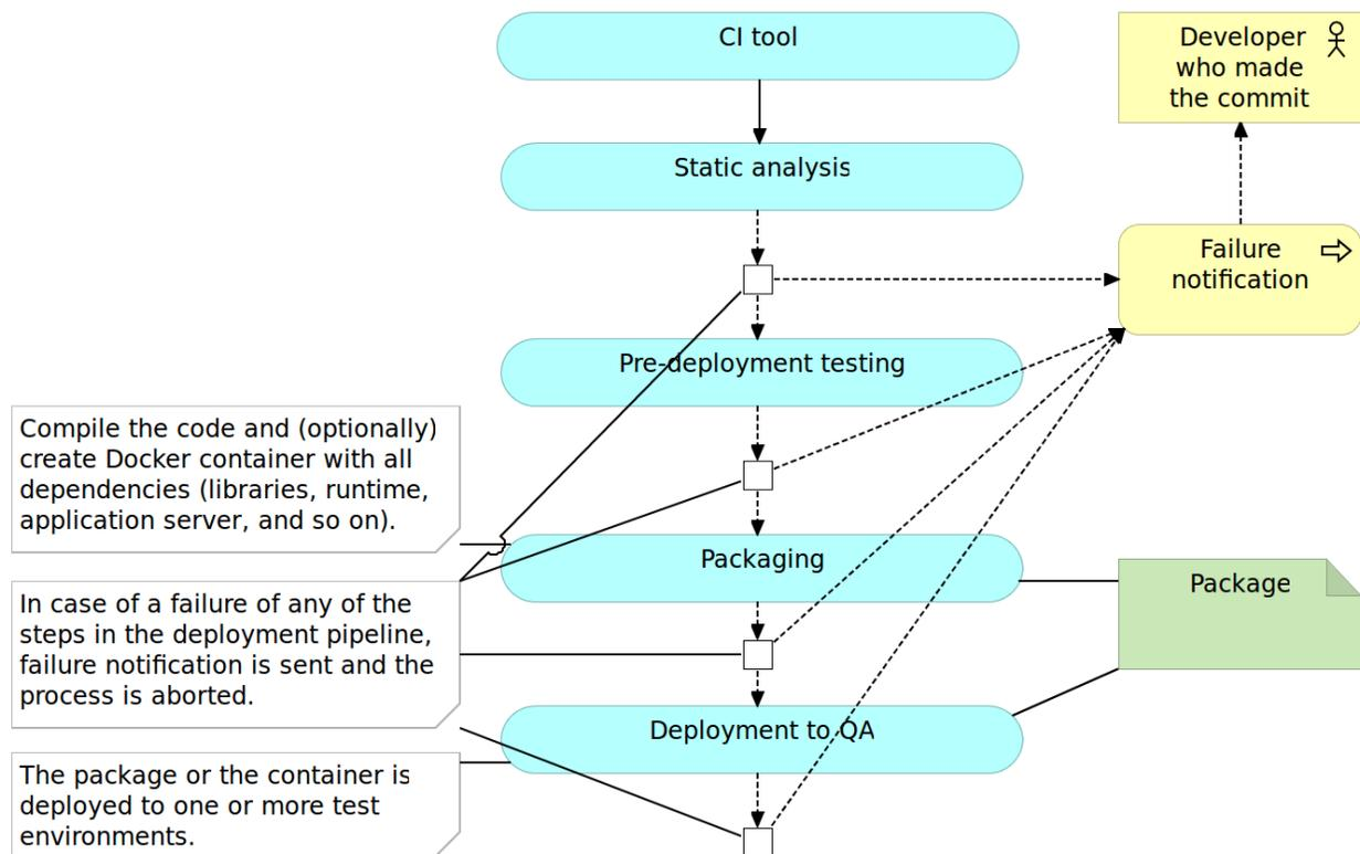
Figure 2-4: Continuous integration pipeline: packaging and deployment
