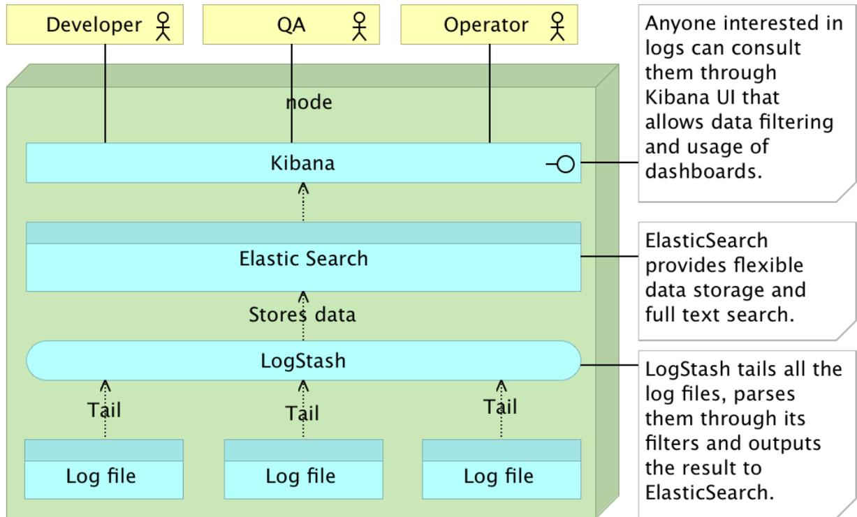
Figure 16-02: ELK stack running on a single server
