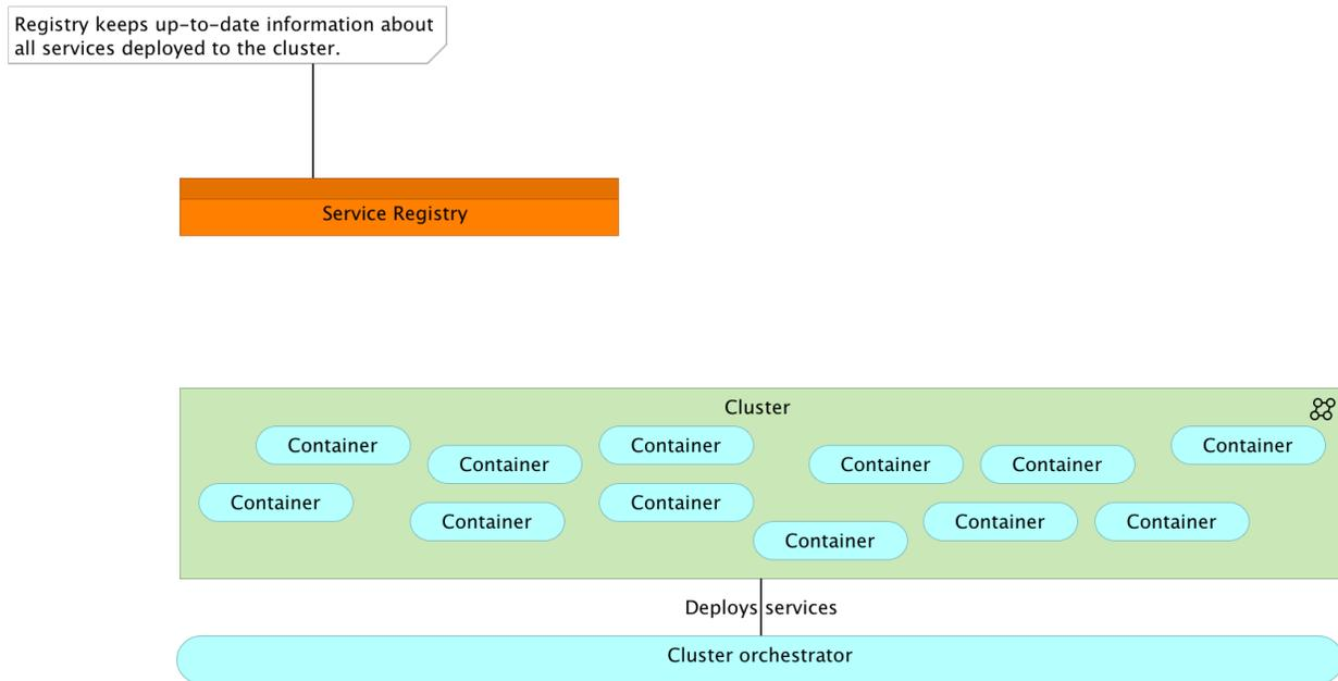
Figure 15-07: Self-healing system architecture: Primary requirement for monitoring the state of the system is to have the information of the system stored service registry
