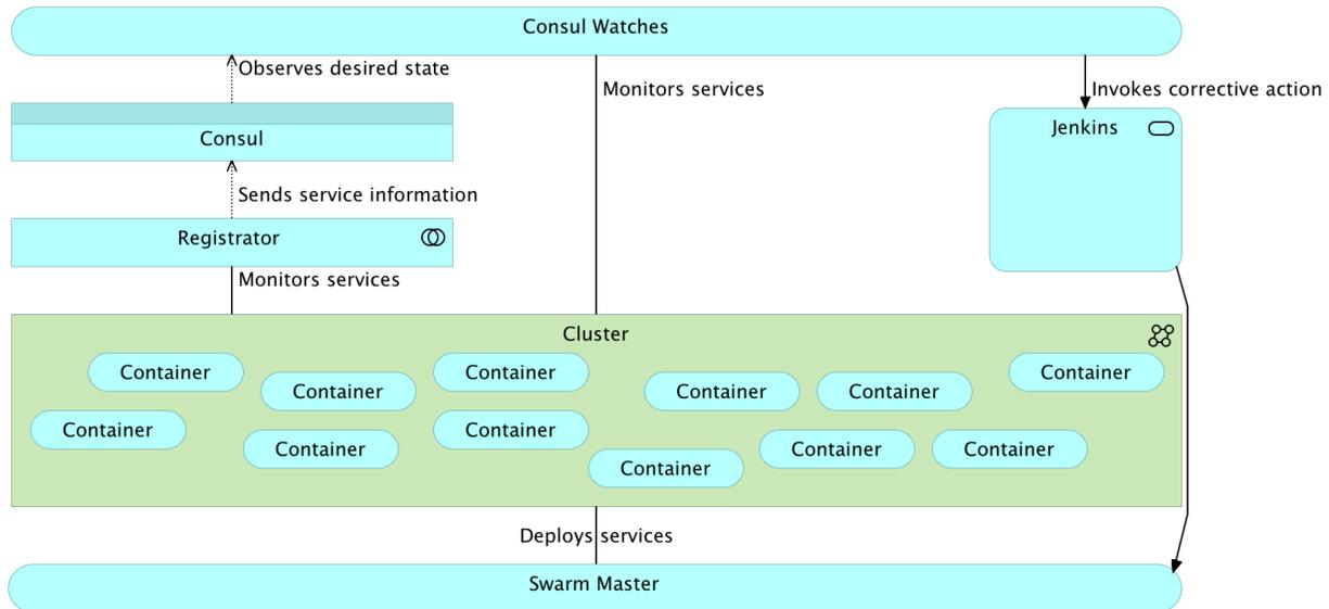
Figure 15-13: Self-healing system architecture: One of the combinations of tools
