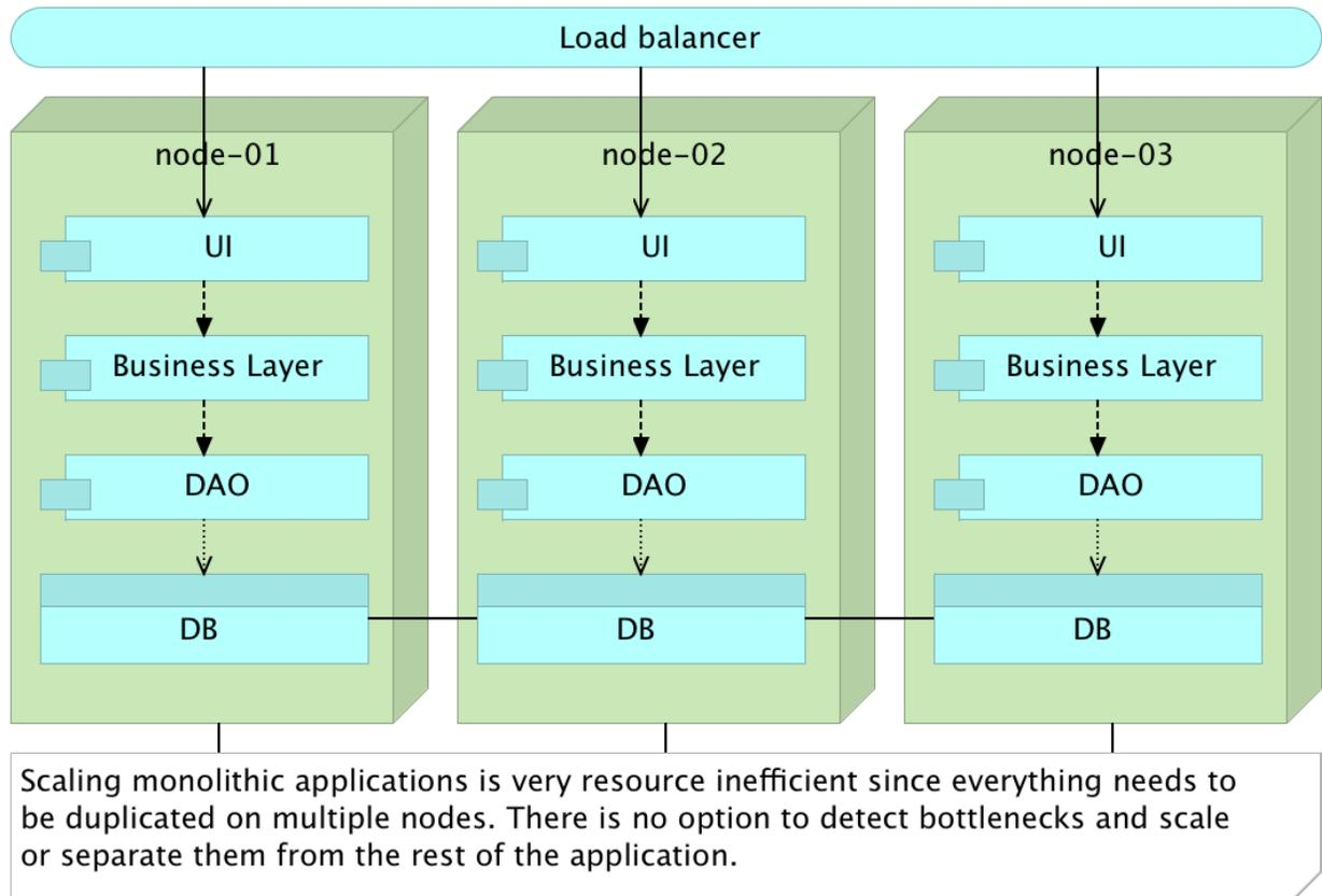
Figure 14-2: Monolithic application scaled inside a cluster
