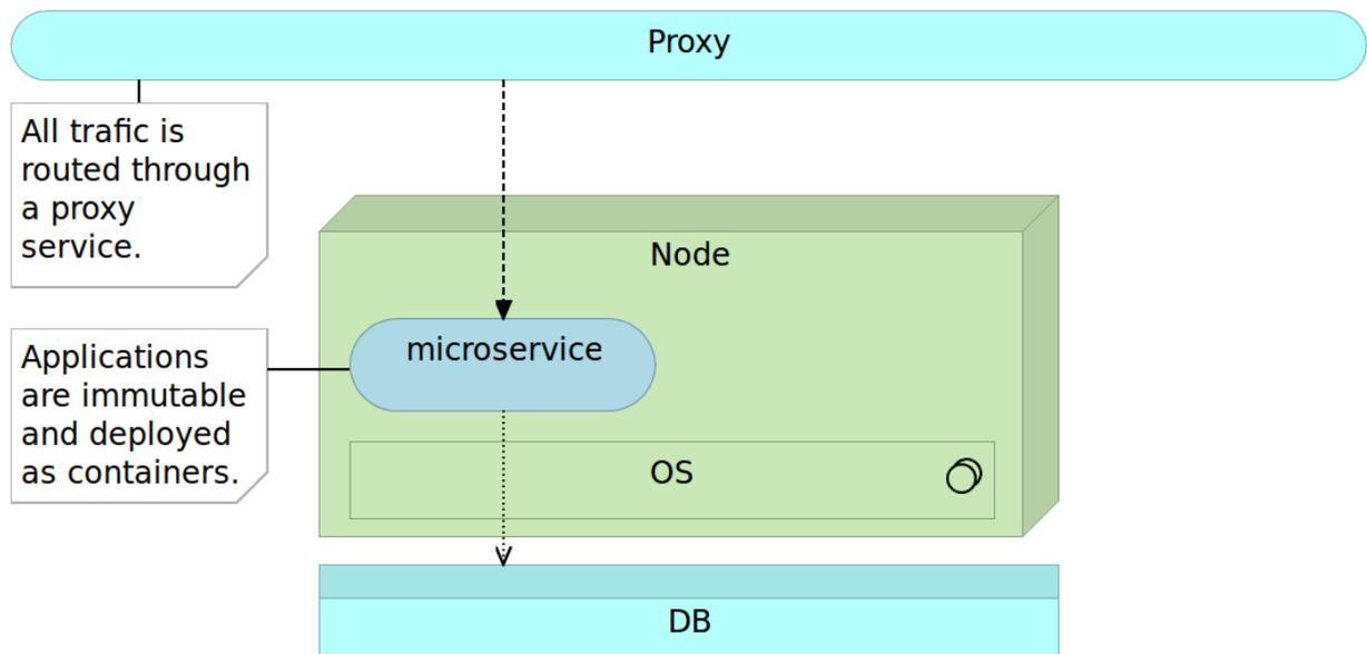
Figure 13-2: Immutable microservice deployed as a container
