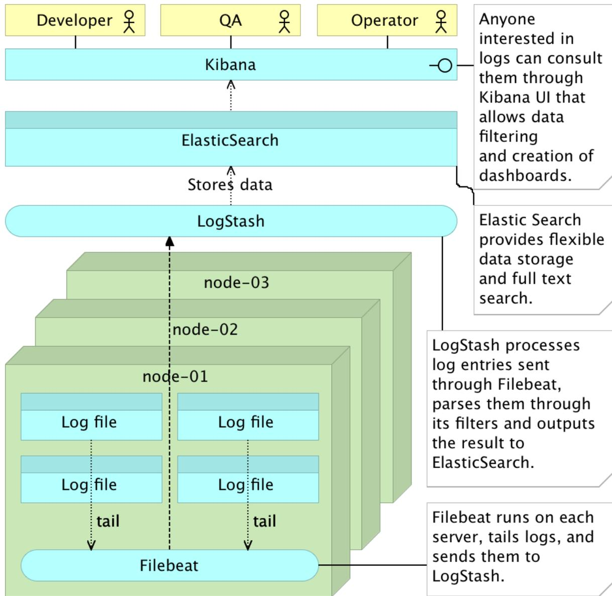
Figure 16-03: ELK stack running on a single server with Filebeat distributed to the whole cluster
